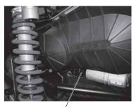
Rear Prop Shaft Grease Fitting
